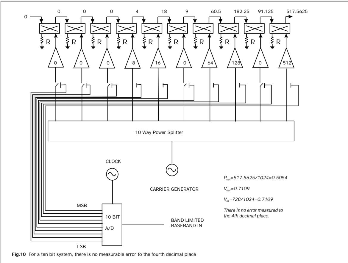
Figure 10 shows that for a ten bit system, where there are 1024 discrete amplitude steps, the significance in the choice of the carry value from the left is insignificant whether it represents a logic one, zero or any value in between.
