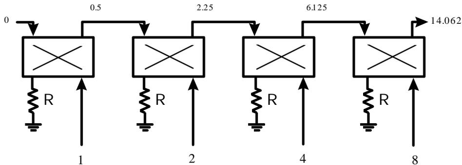
**Fig.4.** With the “carry power” from the left fixed at 0, the power lost in all reject loads is  $15.000-14.062=0.938$  which is only 6.25%.
