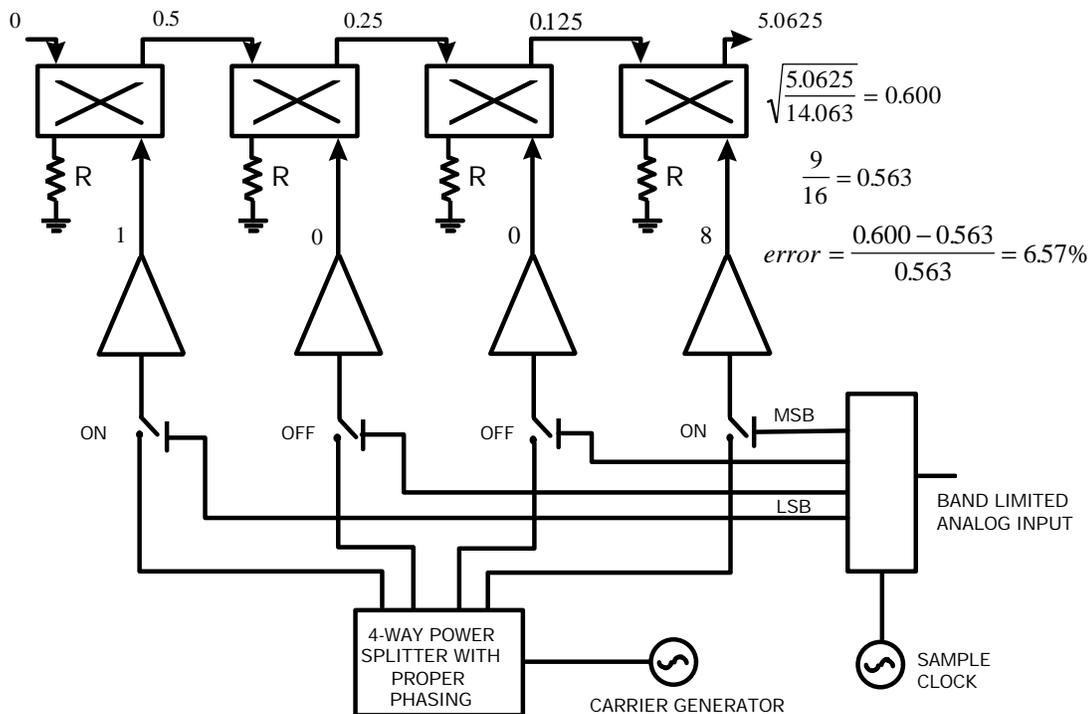
**Fig. 9.** For a sampled baseband waveform at 9/16th of its maximum, or 9 volts in the example, the four bit output power is calculated to be 5.062 watts out of a possible 14.063 maximum for an equivalent voltage ratio of 0.600. This corresponds very closely with the modulation waveform at 9/16ths of its peak at 0.5625 with an error of 6.57%.
