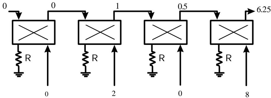
**Fig.5.** With the first and third power sources shut off, using (1) the power at the output becomes 6.25. Since the total input power is  $2+8=10$ , the power lost to the reject loads is 3.75 relative watts.
