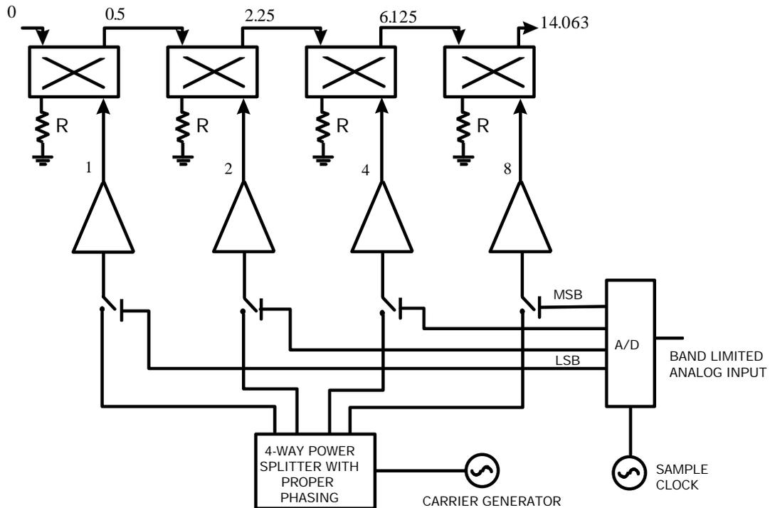
**Fig. 7.** The RF drives of four binarily related carrier power amplifiers are controlled to be ON or OFF by the logic state of the sampled digital baseband equivalent of the analog modulating signal in this four bit Digital Amplitude Modulator.
