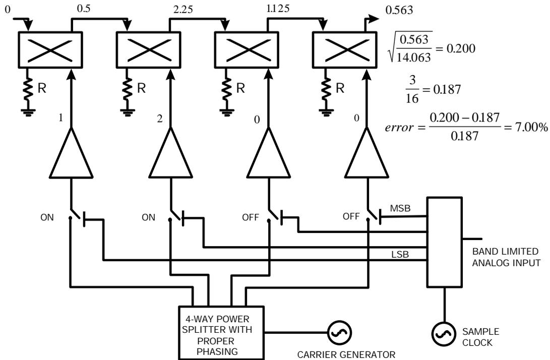
**Fig. 8.** For the sampled signal at 3 volts out of a possible 16, the analog input voltage is 3/16 or 0.187 of its maximum. The square root of the corresponding output power ratioed with the maximum possible, 16 watts, provides 0.200 of its maximum possible output envelope voltage. The error is 7.00% which agrees with that expected of a four bit system.
