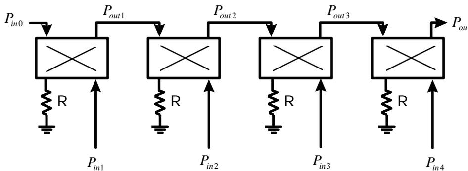
**Fig.2.** Four 3 dB power combiners are arranged so that the output of one feeds the next.  $P_{in0}$  is considered to be from an infinite number of combiners to the left. All of the  $P_{out1,4}$  follow (1) while all reject load powers follow (2).
