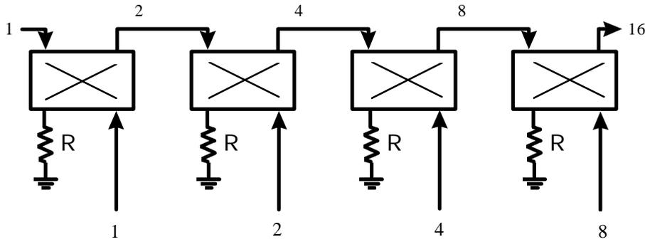
**Fig.3.** Four cascaded combiners are fed with power sources which are double in value as the signal progression moves from left to right. It becomes obvious that the power sources are binarily related in level in order for all power to add to the output without wasting any in the reject loads.
