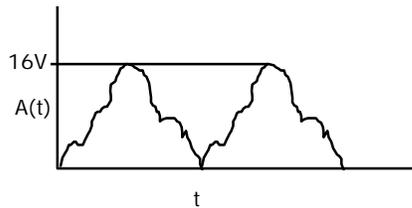
**Fig. 6.** An arbitrary bandlimited modulation waveform, i.e., it is periodic with maximum possible amplitude of 16 voltage units.
