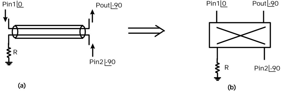
**Fig.1.** For a 3 dB coupler, when  $P_{in1}$  has the same value as  $P_{in2}$  and the voltage vectors are 90 degrees out of phase, as shown, all power adds to  $P_{out}$  and no power is lost in  $R$ . Schematically the hybrid coupler is shown in (b).
